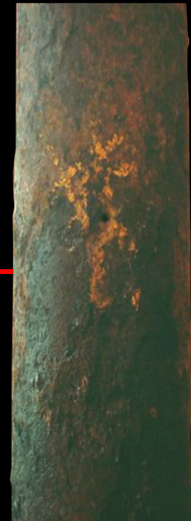
Photo of Corrosion & Hole in Surface Casing @ 6'
