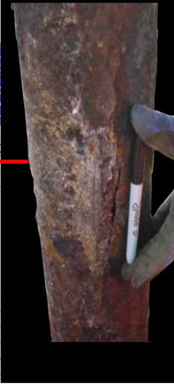
Photo of Corrosion & Crack in Surface Casing @ 5'
